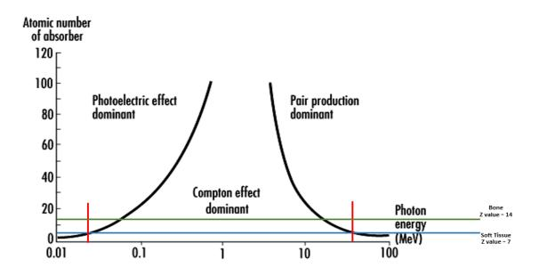
Figure 2.13: Predominating (Most Probable) Interaction vs Photon Energy for Absorbers of Different Atomic Numbers <sup>(44)</sup>
