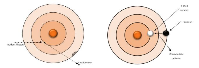
Figure 2.10: The Photoelectric Effect (30, 39)
